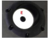
⑦ Screw the plastic reflection plate "E" onto the shaft and tighten the assembly until the plate cannot be turned any further.
