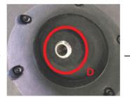
⑥ Insert the second felt "D" onto the shaft as shown.
