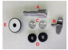
The clutch is assembled from the seven parts shown in the image.
